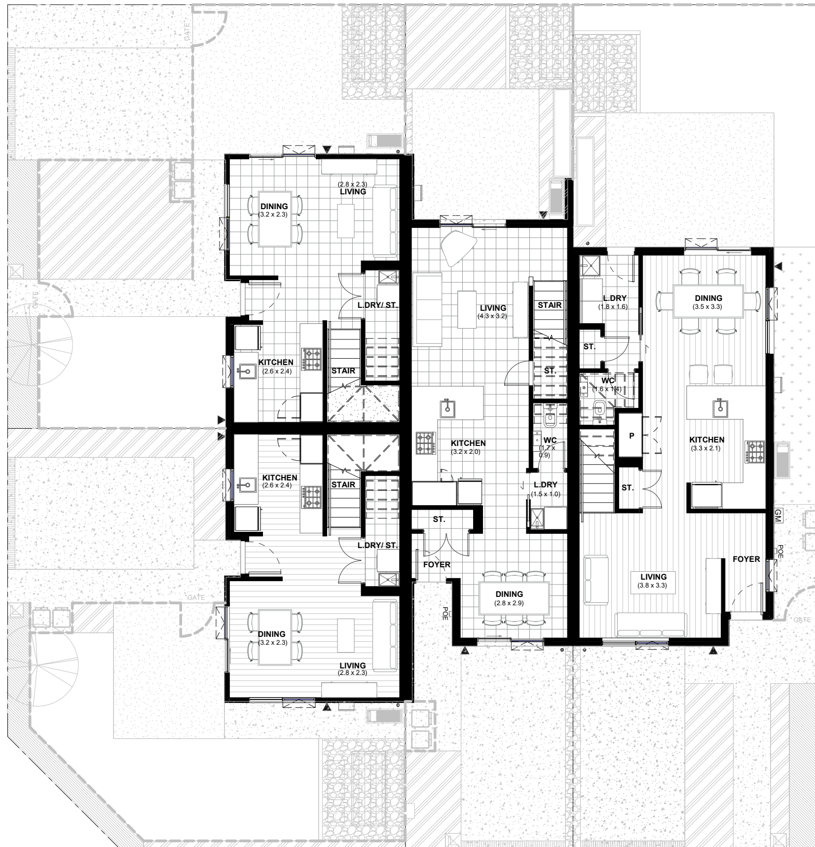
LOT 109 GROUND FLOOR PLAN 26 KATIKATI DRIVE, MANUREWA Floor Area - 70m 2 Site Area - 115m 2 Ground Floor - 35m 2 First Floor - 35m 2
