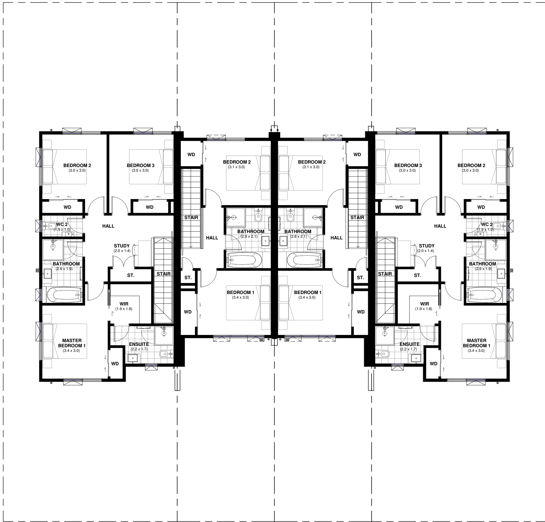
LOT 26 FIRST FLOOR PLAN 191 BROWNS ROAD MANUREWA Floor Area - 140m 2 Site Area - 193m 2 Ground Floor - 68.5m 2 First Floor - 71.5m 2
